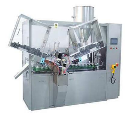
This machine can be used for filling cream and liquid materials, and it is characterized with firm filling and high precision of dosage. The three functions of filling, sealing and batch embossing can be completed automatically. It's widely used in pharmacy, daily chemical, food, chemical industries, (e. g., ) pharmacy cream, hair color, toothpaste, leather oil, glue, nanp-epoxy adhesive etc.
