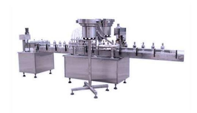
This alcohol filling line is mainly used for filling, capping and sealing 100-500ml alcohol bottles. And it integrates filling and sealing into one body. It is mainly made up of filling machine and sealing machine.
