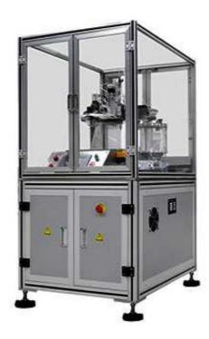
This filling machine for blood collection tube is used for additive spraying.
