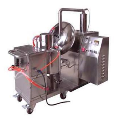
This machine is used to carry out sugarcoating and film coating to the core of Chinese traditional and Western medicine tablets. It integrates strong power, weak power, hydraulic and pneumatic. It is new type equipment improved on the basic of original common type sugarcoating machine.
