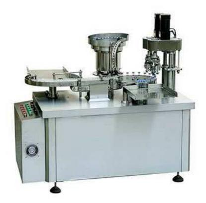
BKGL Automatic chuck capping machine for the application of plastic/glass bottles capping. The machine is composed by a load turntable, conveyor, bottle index wheel, cap unscramble, cap chute &placer, cap crimpling system. The bottle loading/unloading through conveyor manually, or automatic directly from a production line. It is designed and made accordance to GMP regulation.
