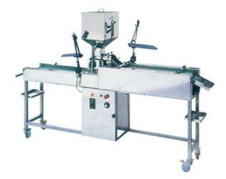
KW-106 inspection machine is designed and used for inspecting capsule or tablet which is spotty, broken. Or not standard by vision through mechanically rotating the capsule over 360 degree or turning the tablet from one surface to the other surface. Inspection can be easily determined.
