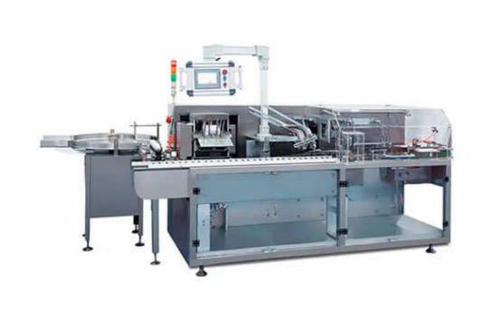
This product is suitable for the packaging of round and shaped bottles and similar items. It can automatically complete the folding of the manual (1-4 fold), carton opening, packing of goods, printing batch number, sealing, etc. Heating the melt sealing device function. It adopts PLC control, photoelectric monitoring of various parts of the action, abnormality during operation can automatically stop showing the cause, in order to eliminate the fault in time.
