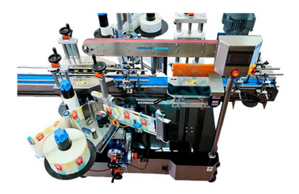
All parameters are adjustable via buttons on the microprocessor, like label length adjustment, label positioning etc. For the conical bottles; the label angles adjustment system is standard on all the machines. The chassis are made of AISI 304 SS, easy mounting and compact design competitive prices.
