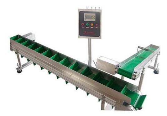
The vacuum conveyor machine is suited for various granule in food convey to machines or tanks by vacuum. adjustable setting of running time and speed, and no limit convey amount. Convey function can be adjust by time or by sensor automatically. According with the heath standard material contact parts made in SS304.
