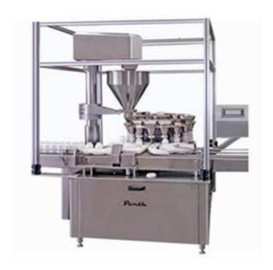
Automatic Dry Syrup Powder Filling Machine is compact machine used for filling of the Dry Syrup in the bottles and is most ideal for wide application in Parma Industries. It is built on strong and robust powder coated M.S. Angle frame Pipe Structure encompassed with S.S.304 hairline prefinished coverings.
