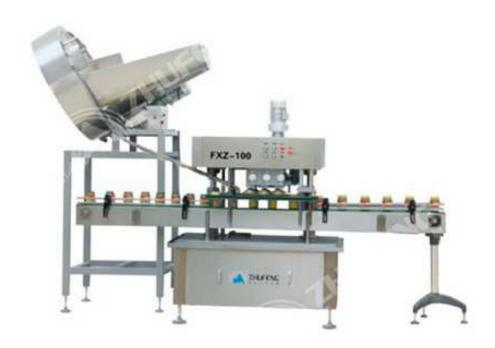
This machine is special use for wide-mouth bottles capping with screw cap, such as fermented bean curd bottles, pickle bottles, flesh bottles. The machine use straight into the bottle, can automatically arrange lid, sleeve lid and capping. Operation simple, production speed fast, the machine also has a back lid function, it is a multi-purpose machine.
