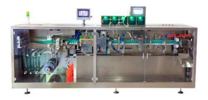
This machine is a kind of smaller type liquid filling and sealing machine, it's suitable for small batch filling in pharmaceutical, pesticide, cosmetic, nutrition etc. field, it's widely used for filling oral liquid, perfume, liquid health care product etc.
