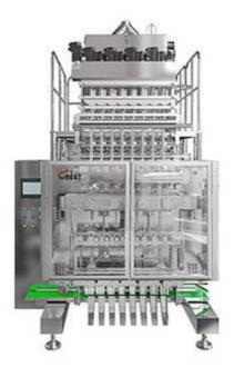
The stick pack multilane packaging machine is suitable for the packaging of all types of products in batch production, such as milk powder, drinks, medicines, health products, condiments, and so on. Adapt to a variety of product specifications, can make various seal patterns and shapes.
