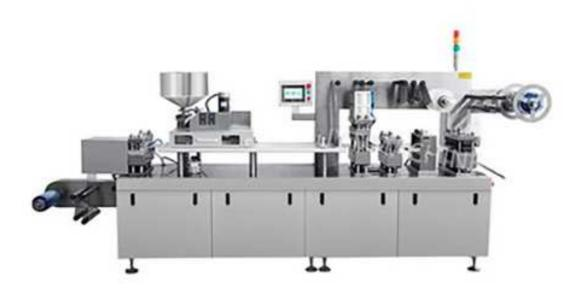
The machine integrates ten functions such as coil uncoiling, aluminum-plastic feeding, blister forming, filling, waste recycling, heat sealing, batch number printing, mesh indentation, sheet blanking, finished product counting, etc. The finished product is well sealed and safe health.
