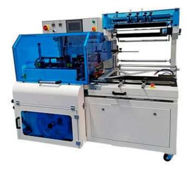
The full-automatic L-Bar sealing machine uses the conveyor belt to automatically operate the product into the folded POF heat shrinkable film. After sealing, the product is heated through the heat shrinkable channel to achieve the effect of sealed packaging.
