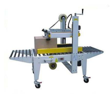
This machine is for the soft cartons, multi-layer carton boxes and daily used cartons, it is usually installed at the beginning of the cartons fill and seal packing lines, to feed the formed cartons and to open and form the cartons one by one to service for the next steps. Its speed decides the whole line speed too, so it is a very import machine.
