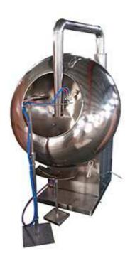
Chinese water chestnut-type coating machine is mainly used for the pharmaceutical industry in the compaction of the tablets, pills, and coated particles can also be used in the food industry in the mechanism or candy coating.
