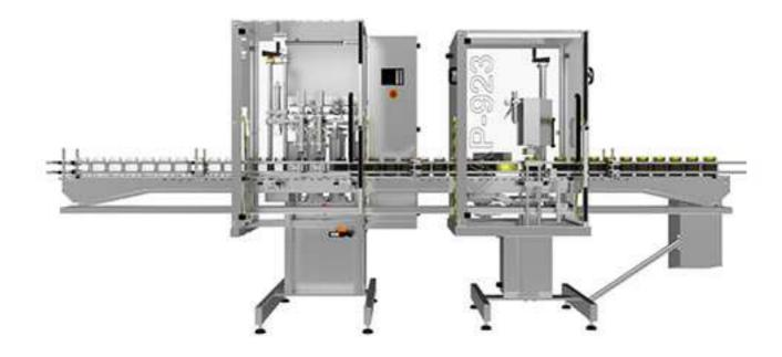
This automatic filler is designed to fill liquid, semi liquid, viscous (paste) and products with particles into the glass and jars & bottles.
