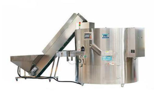
This machine adopts advanced technology, PIC intelligent control, and this machine does not change the mould can arrange for size similar and different shape plastic bottle, could use detergent square bottle or bottle with handle, and such as shampoo bottles, soy plastic bottles.
