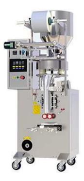
This Automatic Intermittent Vertical Packing Machine Use For Aluminum Plated Plastic Film Packaging is suitable for food particles \* powder \* liquid \* sauce body and other items of measurement packaging
