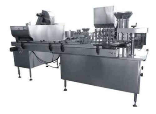
This cosmetic filling machine is specially designed for the unscrambling, conveying, filling, and capping of small plastic bottles. Its main components include unscrambler, conveyor belt, filling machine, and capper.
