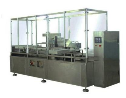
AGF8- ampoule machines is researched and manufactured by our factory, it is applicable for filling and sealing of 1ml, 2ml, 5ml, 10ml and 20ml ampoules. The machine can either be used as a single machine, or be used together with sterilized tunnel oven and ampoule ultrasonic wave washing machine.
