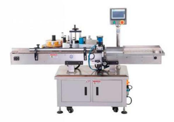
At the beginning of the working process, the bottles are fed to the labeling machine at a constant speed on the conveyor belt. The mechanical fixing device separates the bottles by a fixed distance, and pushes the bottles along the conveyor belt. The mechanical system of the labeling machine includes a driving wheel, a labeling wheel, and a reel.
