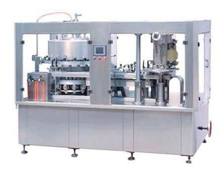
The machine is for the isobaric filling and sealing of carbonated drinks like beer and beverage which is packed by pull-tab aluminous cans, tins or PET plastic cans. It adopts mechanism, electric and pneumatic control technique, having the characteristics of automatic can-feed, automatic aluminum top falling, and no filling and sealing.
