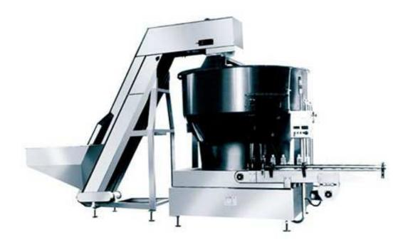
LPJ serial full-automatic bottle unscrambler is the support equipment for the soft beverage filling equipment, applicable for the orderly arrangement of messy PET bottles and the delivery of them to production line.
