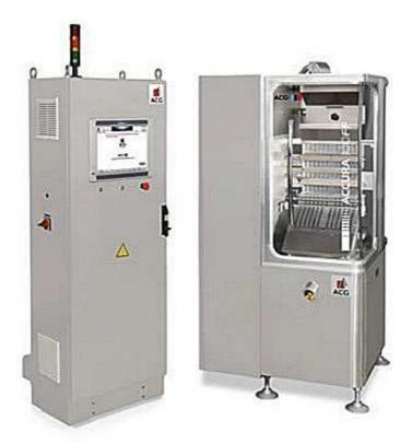
Accura, a series of 100% capsule check withers can be easily integrated with existing high speed encapsulation machine for pre or post fill check weighing. Enhancing the quality of capsules the Accura ensures that every capsule is well within compliance limits. The Accura's measuring capabilities are enhanced by pioneering EMFR load cells from Wipotec, Germany which are sensitive to variation of 1 mg. The group load cell technology along with the compensation cell ensures accuracy of +/- 2 mg
