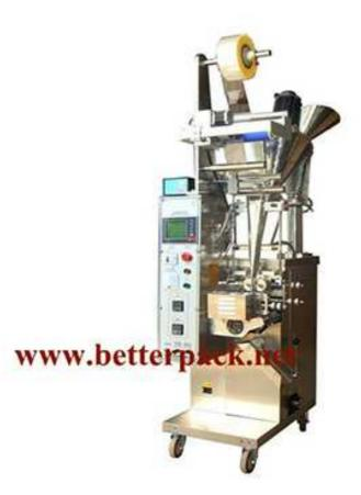
This machine is quite suitable for the 3 side seal package of powder such as spice powder, coffee powder, milk tea powder, curry powder, chocolate powder and other kinds of powder in food, chemistry and medicine. It is also can be used to pack granule or liquid by changing the measuring and filling parts.
