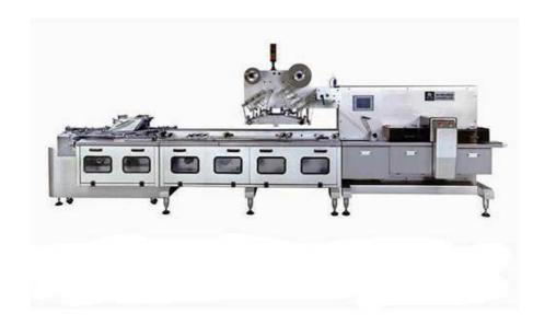
Most of the time, this system is generally composed of at least one automatic distribution device plus several set of feeding mechanisms. From the front-end production, the chocolate or related products maybe come without order. The distribution device can make all the products in good order before entering feeding system.
