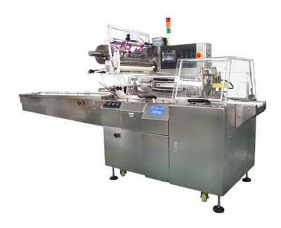
Automatic Reciprocating packing machine with angle folding device is suitable for packing regular objects such as biscuits, pies, bread, fresh fruits & vegetable, instant noodles, drugs, daily appliances, industrial parts, paper boxes, plates, etc.
