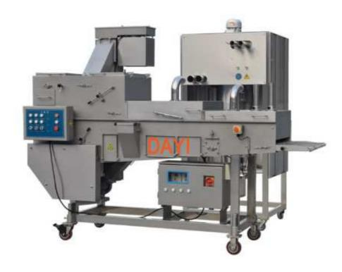
This Patty breading machine can evenly coat the meat like chicken, beef, pork, and seafood by outpouring the crumb from the hopper when the products is carried by the belt passing under it. For the bottom coating, there is a layer of crumb on the lower belt. Also there is a roller pressing sytem to press tightly the crumb onto the surface of the food and the thickness of crumb can be regulated by this unit too.
