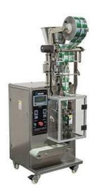
This machine can fully make the automatic package for all kinds of grain or granules, like sugar, rice, salt, beans, peanuts. etc.
