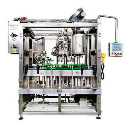
This machine is the latest design of the beer filling machine 3 in 1 type. It adopts external filling valves; all filling valves were hung on outside of the beer tank, which has no contact with the beer inside. This can guarantee the beer won't have any bacteria infections reliable than the original design.
