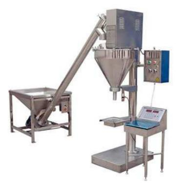
This powder auger filler machine adopts screw filling and electronic weighing feedback measurement methods, combined with the microcomputer control, this auger filler machine has the function of automatic quantitative, automatic filling, automatic error correction, counting, clear material etc.
