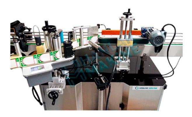
All parameters are adjustable via buttons on the microprocessor, like label length adjustment, label positioning etc. For the conical bottles; the label angles adjustment system is standard on all the machines. The chassis are made of AISI 304 SS, easy mounting and compact design competitive prices.
