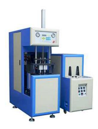
WBS-2 Semi-automatic Bottle Blowing Machine is suitable for producing plastic containers and bottles from 10-2000ml. It is widely to produce Soda bottle, mineral water, carbonated drink bottle, pesticide bottle, oil bottle, wide-mouth bottle etc.
