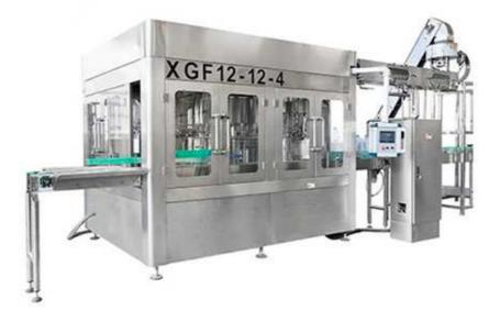
This machine works harmoniously with air-conveyor belt, It holds the bottles by the neck, thus, reducing the possibility of bottles falling over during conveying process. This machine is used to fill still water into pet bottle and with screw caps capping function.
