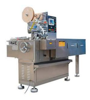
This Bouillon cube Side seal Wrapping machine is used to pack all kinds of cubes, like bouillon cubes, sugar cubes, and green bean cake etc.
