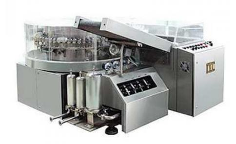
ACQ80 (60) (40) Ultrasonic wave washing machine is specially designed for automatic washing of various kinds of ampoules. This machine is mainly applicable for the washing of 1ml, 2ml, 5ml, 10ml and 20ml ampoules. This machine is of vertical rotation structure, it uses mechanic hand to clamp and overturn the bottle, and it uses ultrasonic washing and water-air alternation spray to wash the bottle one by one.
