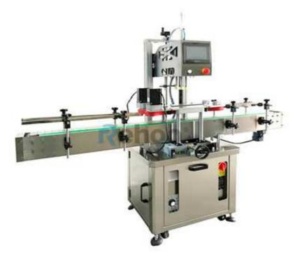
The linear capping machine has high capping speed, high pass rate and easy operation. Applicable to different bottle-shaped screw caps in food, pharmaceutical, daily chemical, pesticide, cosmetics and other industries. Four speed-regulating motors are used for cap feeding, bottle clamping, conveying and capping. The machine has a high degree of automation, good stability, and easy adjustment. No spare parts are required when changing the bottle shape or cap, and it can be done by adjusting.
