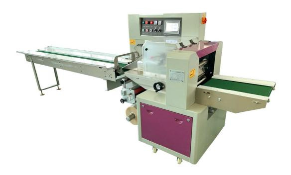
Horizontal flow packaging machine is a three-servo machinery, which can pack different products, such as plates, bread, sausages, fish, ice-lollies, soft candies, fresh fruits etc.
