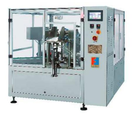
FFT-G rotary bag given packing machine which replaces the manual packaging, the packaging machinery automatically catch pre-made bag, date printing, bag opening, according to metering device signal measurement and fall material, sealing, output. Automatic rotary bag given packaging machine has advantages of sealing beautiful, high capacity, good sealing performance, more and more favored by the customers.
