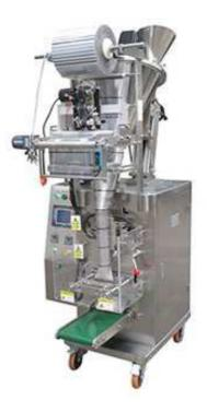
Automatic Stick Milk Powder Packing Machine are widely used in food, medicine, feed, veterinary drugs, chemicals, additives, desiccants and many other industries. The whole machine is designed in accordance with GMP standards.
