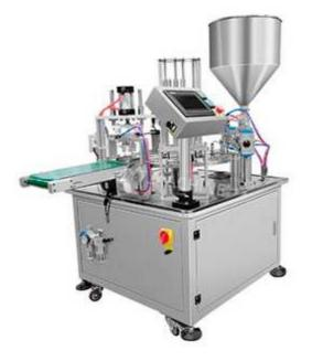
Rotary type liquid cup filling sealing machine is suitable for packaging a wide range of liquid sauce and paste products into pre-formed containers of various size and shapes. It can automatically finish the process of falling cup, filling, sealing and outputing finished products.
