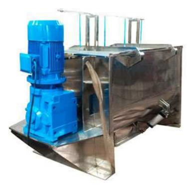
This Mixing Machine is widely used in chemical industry, plastic, rubber, food, medicine, polymer, building, fireproof materials and other particles, powder, liquid material mixing. Working Method: This horizontal ribbon Mixer Machine is arranged on the transmission main shaft double-layer spiral blade, the external blade will transport the material to the middle, the internal blade will transport the material to the outside.
