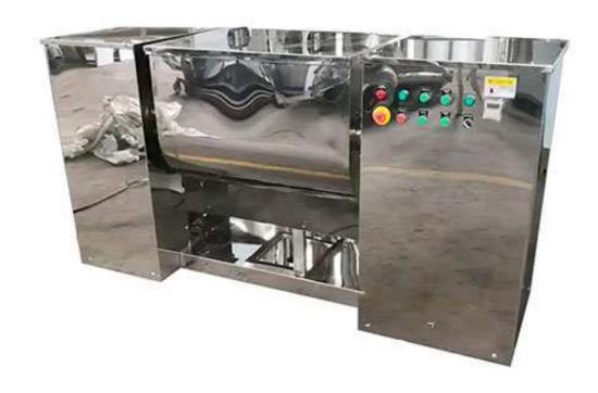
Main Application This Mixing Machine is used for mixing powder or wet materials to make main and auxiliary materials of different proportions mix evenly. The Mixer Machine is made of stainless steel where it contacts with materials. The gap between pulp leaves and barrel body is small and there is no dead Angle in mixing. Sealing device is set at both ends of stirring shaft to prevent material from exuding. Widely used in pharmaceutical, chemical, food and other industries.
