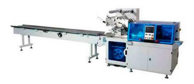
ZF-Z240/ZF-Z360 mainly used for fully sealed shrink packaging of single product. The packaging speed can reach 80-100 pieces per minute. Packaging effect is very beautiful. Feeding system can be connected to existing production line to improve production efficiency.
