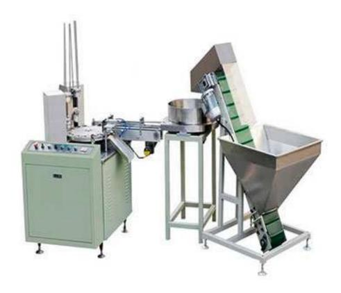
This cap lining machine is widely used in food and pharmaceutical caps, in which it is necessary to insert the double-layer pads (aluminum foil and paper) into the bottom of the caps. The specially designed mold can produce a pulled piece on the aluminum foil to be easily opened.
