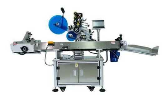
NY-817F automatic paging and labeling machine can work for all kinds of objects with plane, flat surface such as card, bags, books, unshaped boxes, cartons, paper, pouch and other packaging bag etc. Adopts automatically separate stacks of packaging bags or cards and convey single piece onto the conveyor belt so as to facilitate labeling machine to stick each sticker onto objects and thus reduce the trifles of manual paging to improve labeling efficiency.
