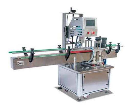
The fully automatic capping machine of our factory adopts electrical combination to control the movement, with high stability. It can lock caps of different shapes and specifications. The speed of the cap locking can be adjusted and the tightness can be adjusted according to different caps.
