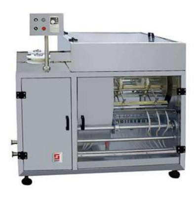
Suitable for all kinds of round and irregular-shaped bottles in various materials from 30ml to 500ml while adopting two-times water washing and one-time air washing to wash bottles inside and outside, which makes the washing process comply with working flow requirement. The machine can also preliminarily dry bottles.
